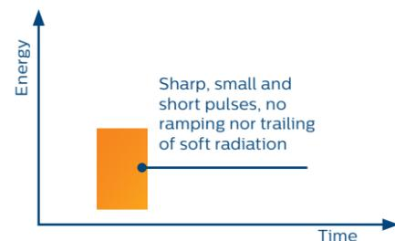
**GCF:** Sharper, smaller and shorter pulses without ramping or trailing of soft radiation, delivers only dose that contributes to the image
