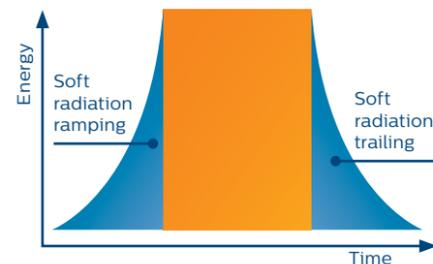
**PCF:** Un-sharp, high and long pulses, with ramping and trailing, creating extra dose for the patient through soft radiation
